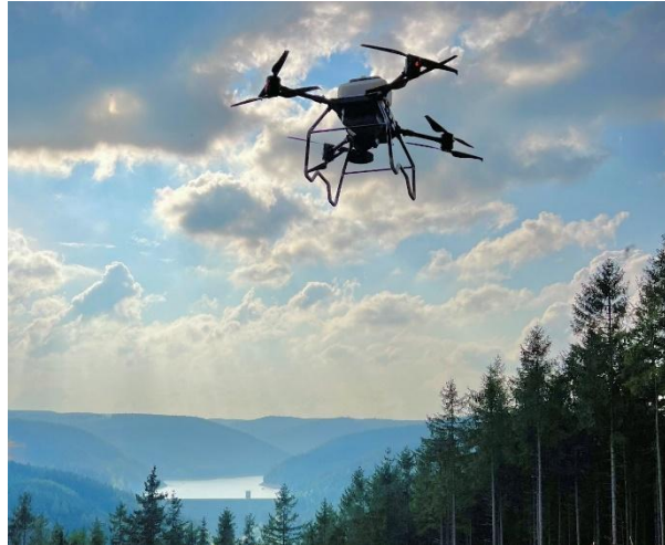
Figure 2. An aerial drone used to efficiently broadcast seed at forestation sites that are remote or of difficult terrain (Photo credit: Skyseed GmbH, Germany).
