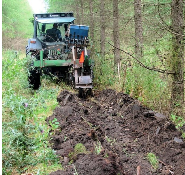
Figure 3. A tractor-drawn mechanical seeder used to prepare the seedbed in a Norway spruce ( Picea abies (L.) H. Karst.) plantation and sow a seed mix of desired species directly into the row of prepared soil (Photo credit: Palle Madsen).
