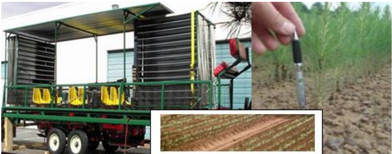
Figure 14. Transplanter designed to plant miniplug loblolly pine seedlings (left) into bareroot nursery beds (insert) and established miniplug seedlings in the bareroot nursery (right) (Grossnickle unpublished data).
