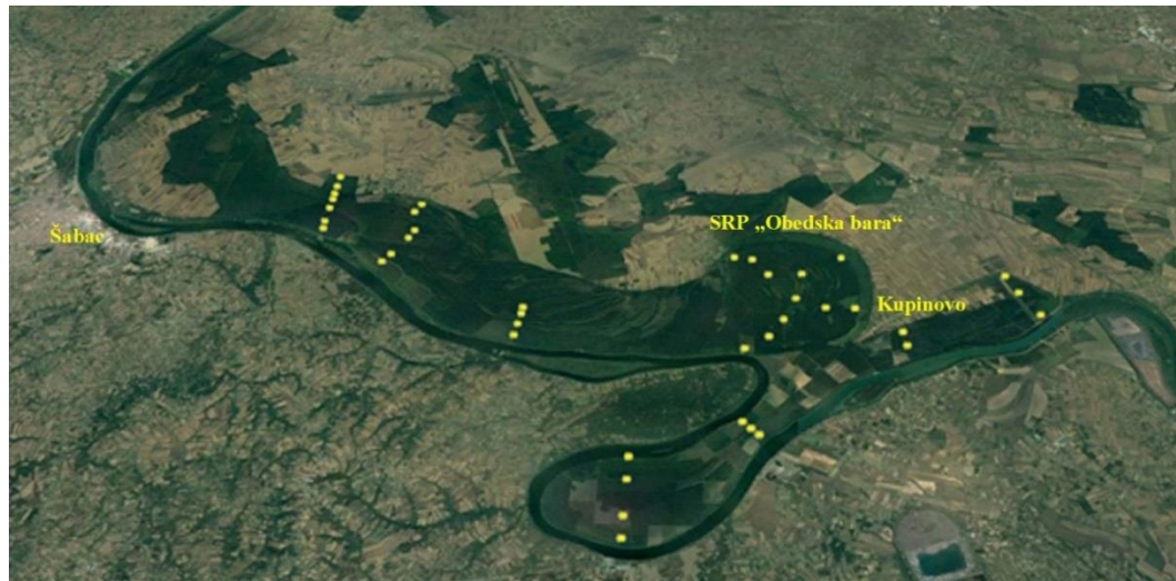
Figure 2. Distribution of piezometers installed at investigated area.
