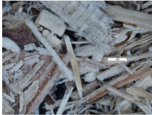
Figure 1. Light microscope image of loblolly pine ( Pinus taeda ) sawdust used for biochar feedstock (1 mm scale shown).
